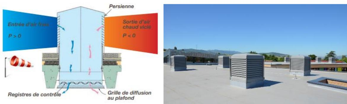
Figure 59 : Tourelle de ventilation naturelle Windcatcher © Kingspan [62]
