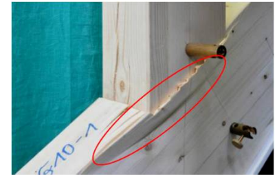
Transverse compression below the joint [1]
