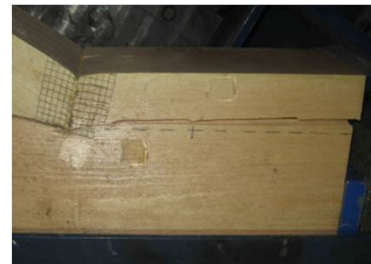
Shear crack at the heel depth [2]
