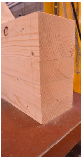
Bending/Shear in the reduced section ( l_{ecc} )
