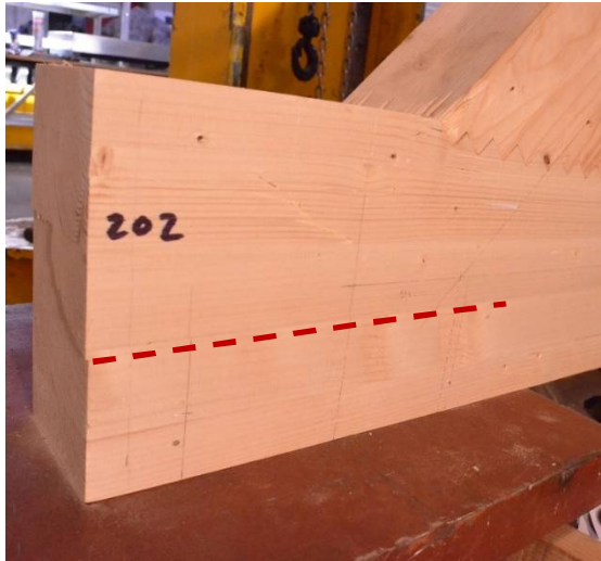
Classic beam shear under transversal compression in the tie beam : final failure in bending
