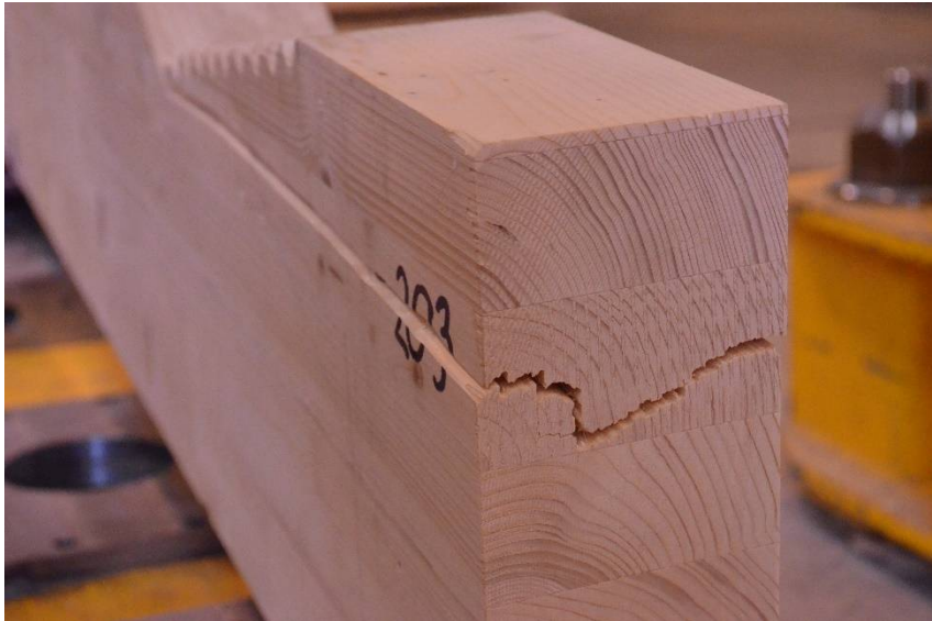
Shear crack at the heel depth ( l_{v,eff} & k_{v,red} )
